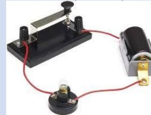
3. A lamp will only work in a complete circuit.
